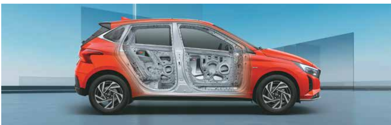
Strong body structure (with AHSS and HSS)
