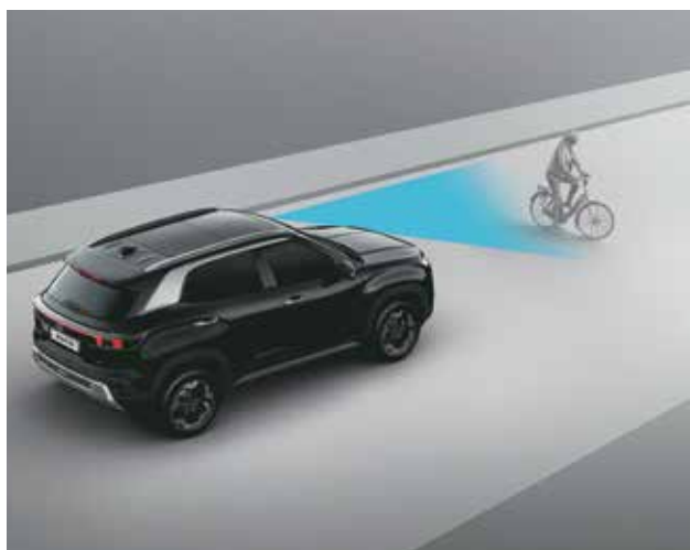
Forward Collision - Avoidance Assist - Cycle (FCA-Cyl)
