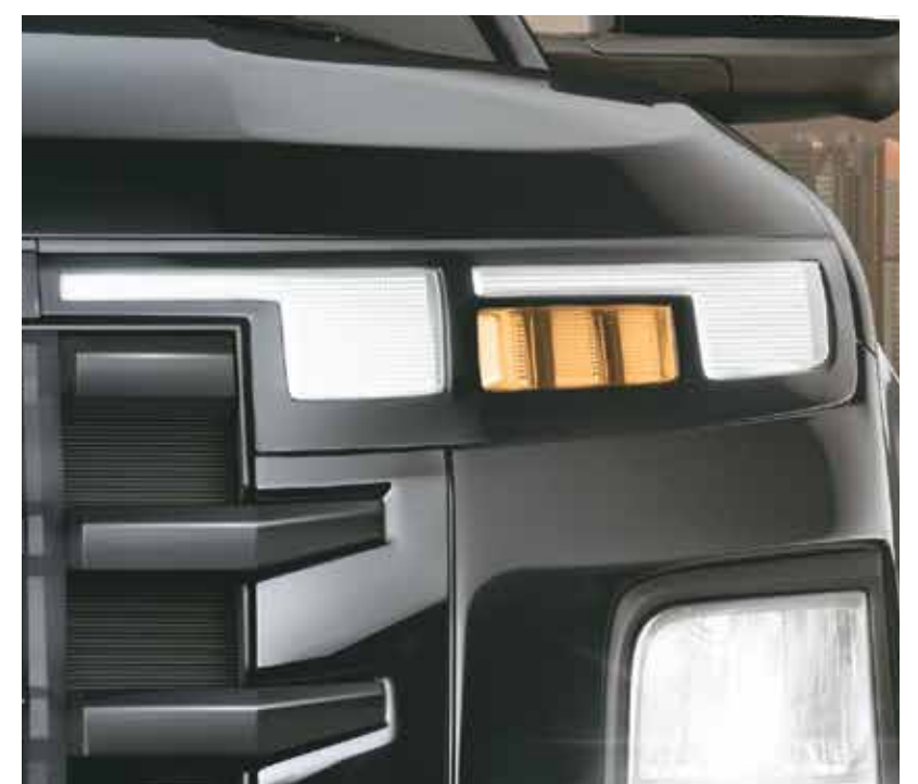
Front turn signal with sequential function
