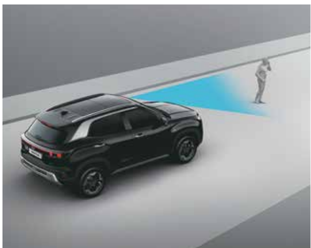
Forward Collision - Avoidance Assist - Pedestrian (FCA-Ped)
